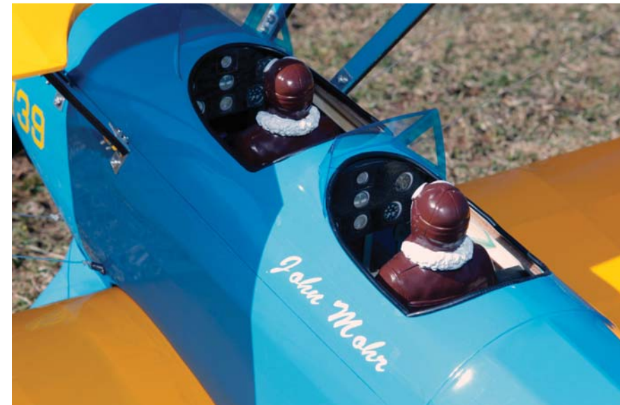
The 1/8 scale pilots fit perfectly in the cockpit, but I had to trim one instrument down and add 1/4-inch balsa stock to the other to get them to fit into the cockpits.
