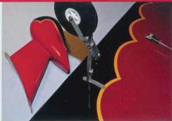
The fiberglass wheel pants cover the shock-absorbing main gear legs for a neat, attractive finish.
