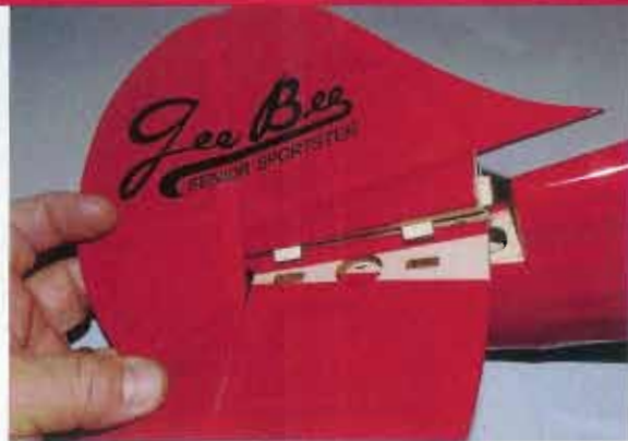
The tail feathers interlock, so the alignment is made sure. Features like this make the Gee Bee Y a fast build.
