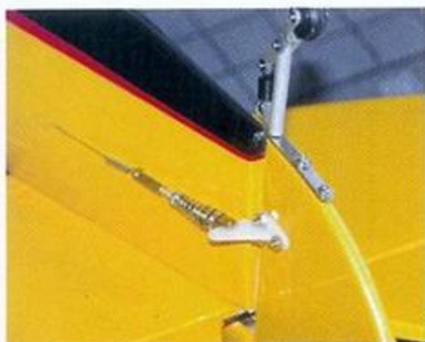
The tail landing gear is held in place with CA and two screws that secure it to the rudder.
