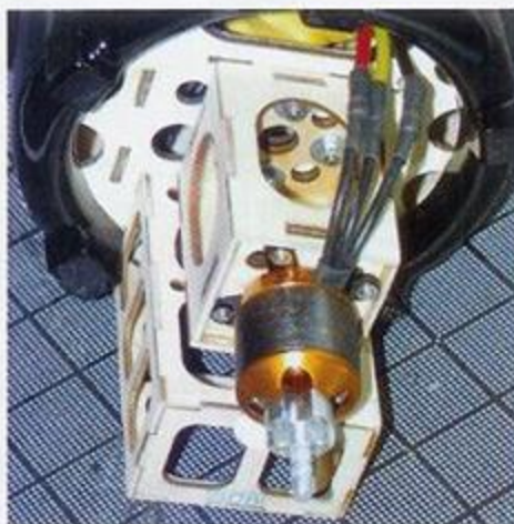
The motor mounts to a wooden frame that in turn is bolted to the firewall of the fuselage.
