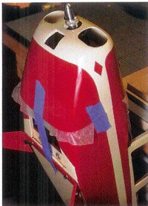
With all the plywood components in place, secure the cowl with tape, and apply epoxy to each mounting tab through the front of the cowl. Be careful not to glue the screws in place.
