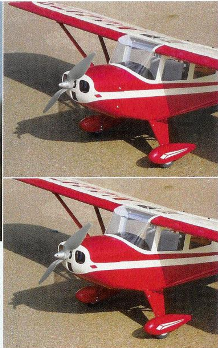
Mounting the cowl with internal screws cleans up the look of a model slightly, and provides much better support for the cowl.
