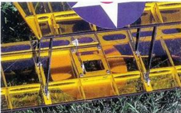
The aileron servos are mounted in the wings for direct linkage and easy installation. The roundels hide them nicely. The scale-like rigging really adds to the appearance of this classic flyer.
