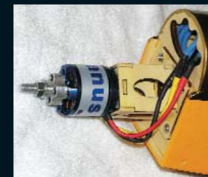
Top: The realistic pull-pull control cables give lightweight positive control to the rudder and elevator surfaces. Above: The kit includes mounts for both glow and electric power systems with proper thrust line all preset. The Uranus motor is available direct from Maxford USA.
