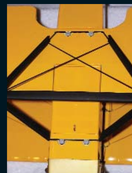
Battery access is through the hatch above the landing gear legs.
