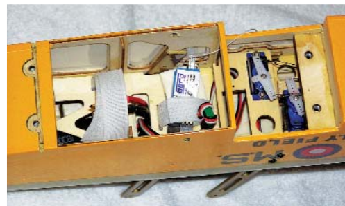
Access to the receiver, and rudder and elevator servos is through the lower wing saddle. Make sure these controls are setup and working properly before assembling the wings to the fuselage. Note the large battery compartment to the left.
