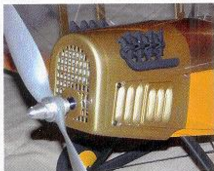
The fiberglass front cowl gives the plane an authentic scale appearance.
