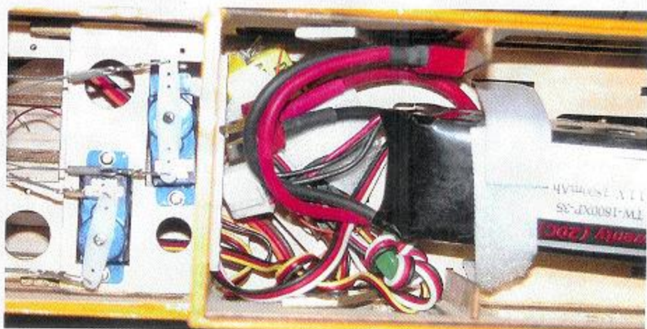
Left: the final setup of all the pull-pull controls gives the tail feathers a unique visual appeal. Below: with the receiver, servos, and battery in place, there is still plenty of room for fingers to install and remove the battery pack.
