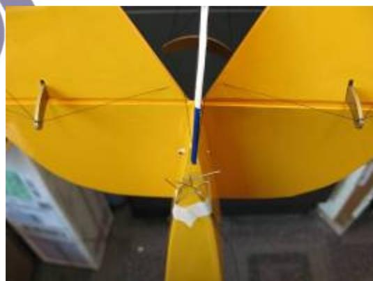
Insert the  $\frac{3}{4}$ " bolt through the three holes. Place a washer and a nut on the bolt and tighten. Do not crush the wood under the screw. Place a small drop of thin CA at the end of the screw and nut.
