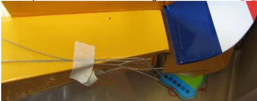
Pin-hole in covering hides the hole for the  $\frac{3}{4}$ " bolt.
